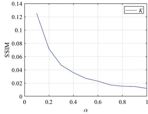
**Fig. 8.** Diagram of SSIM for extracted watermark ( $T = 0.01$ ), averaged for the delay length  $K$  ( $1 \leq K \leq 20$ ).
