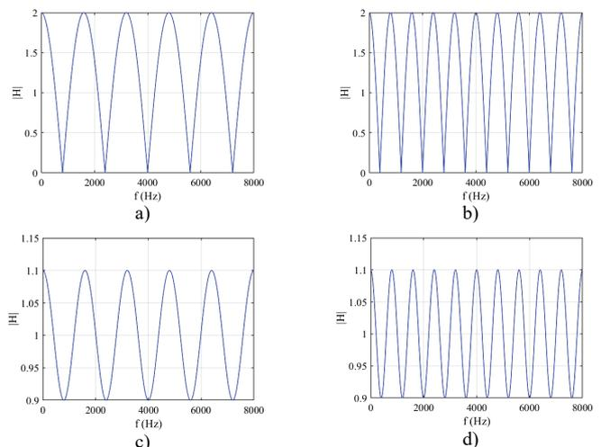
Fig. 2. Amplitude characteristics of Comb filter for: a)  $K = 10$  and  $\alpha = 1$ , b)  $K = 20$  and  $\alpha = 1$ , c)  $K = 10$  and  $\alpha = 0.1$  and d)  $K = 20$  and  $\alpha = 0.1$ .
