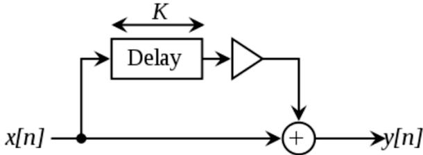
Fig. 1. Block diagram of the Comb filter
