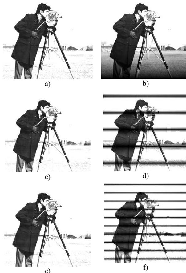
**Fig. 4** Visual appearance of image after applying the Comb filter for: a)  $K = 1$  and  $\alpha = 0.1$ , b)  $K = 1$  and  $\alpha = 1$ , c)  $K = 10$  and  $\alpha = 0.1$ , d)  $K = 10$  and  $\alpha = 1$ , e)  $K = 20$  and  $\alpha = 0.1$  and f)  $K = 20$  and  $\alpha = 1$ .
