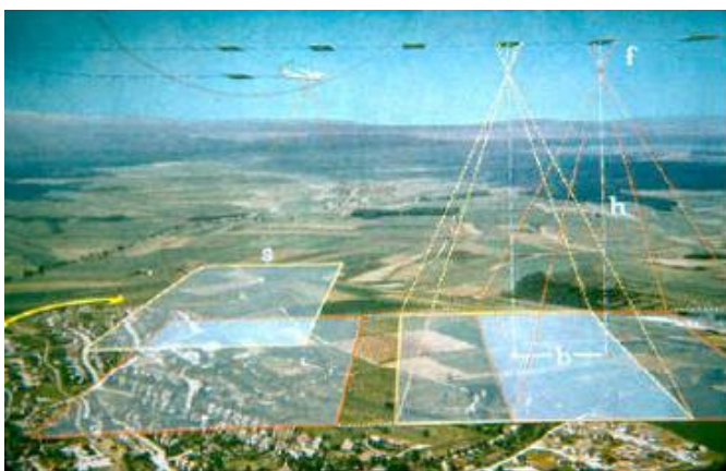
Fig 1. Aerial photogrammetry is done using pictures taken from specially equipped aircraft.
