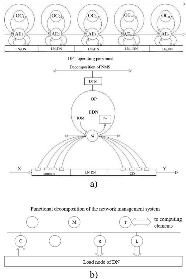
**Fig. 2.** Decomposition of the network management system: a) structural; b) functional; C - collection and processing of information; R - regulation; L - logical control; M - manual input and display of information; T - transmission of information; Pr - processor; IOM - input-output module; OC - object controller; DTM - data transmission multiplexer
