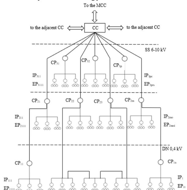
**Fig. 1.** Topology of the lighting control system
