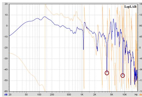
Fig. 5. Frequency response of Selenium 10MB3P loudspeaker (pink noise) LspLAB
