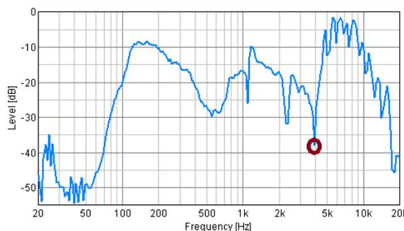
Fig. 6. Frequency response of Selenium 10MB3P loudspeaker (frequency sweep) Realtime Analyzer
