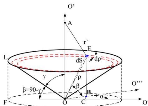
Fig. 1. Geometry of conical piston acoustic transducer
