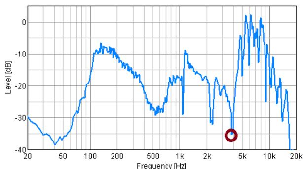
Fig. 7. Frequency response of Selenium 10MB3P loudspeaker (pink noise) Realtime Analyzer
