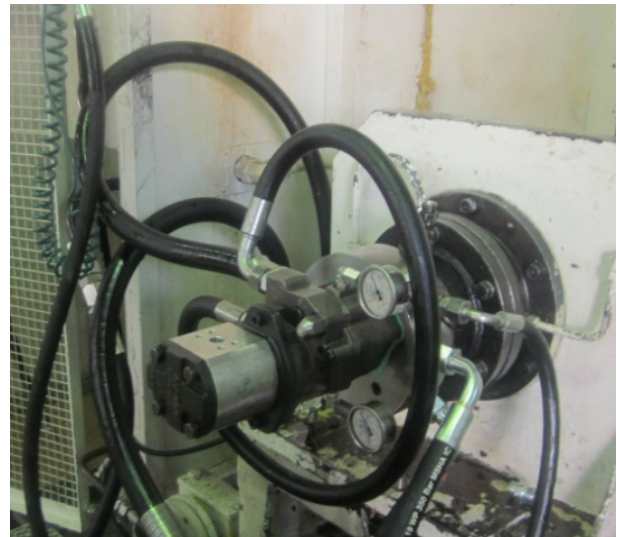
Fig. 5. Connection of gear pumps to test setup
