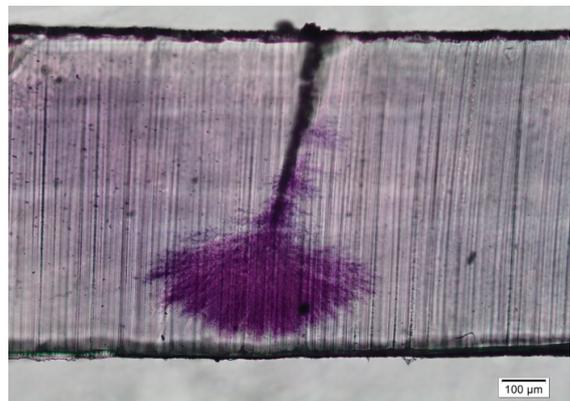
*Fig. 16. Microscope image of vented type water tree (1M, 24 kV<sub>pp</sub>, 3 kHz, 24 hours, 84.2 mS/cm)*
