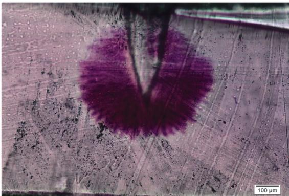
*Fig. 12. Microscope image of vented type water tree (1M, 24 kV<sub>pp</sub>, 3 kHz, 24 hours, 84.2 mS/cm)*
