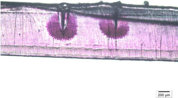
**Fig. 5.** Microscope images of vented water trees (1M, 24 kV<sub>PP</sub>, 3 kHz, 24 hours, 84.2 mS/cm)
