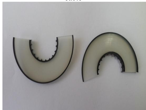
**Fig. 2.** Image of insulator sample taken from XLPE insulated single core medium voltage cable
