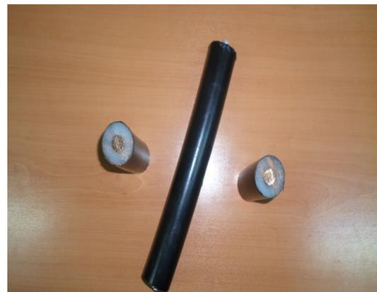
**Fig. 1.** XLPE insulated single core medium voltage cable
