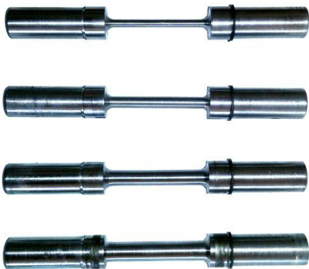
Fig. 2. Steel shaft with different diameter.
