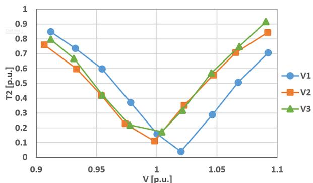
Fig. 5.  $T_2$  at single-phase unbalance
