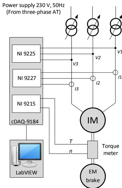
Fig. 1. Block scheme of measurement system
