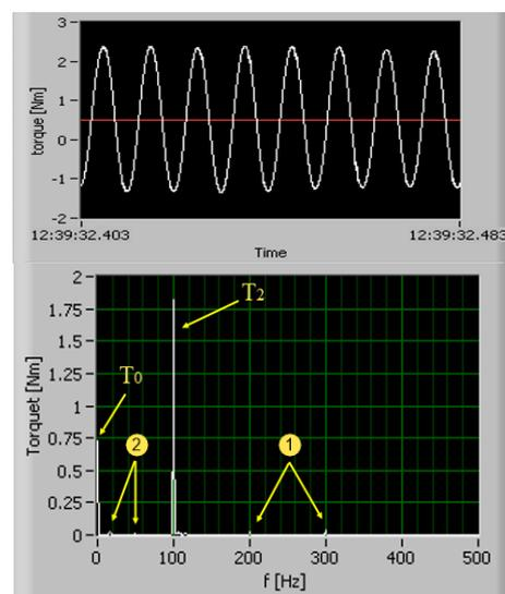
**Fig. 4.** Profile of the torque and its frequency components
