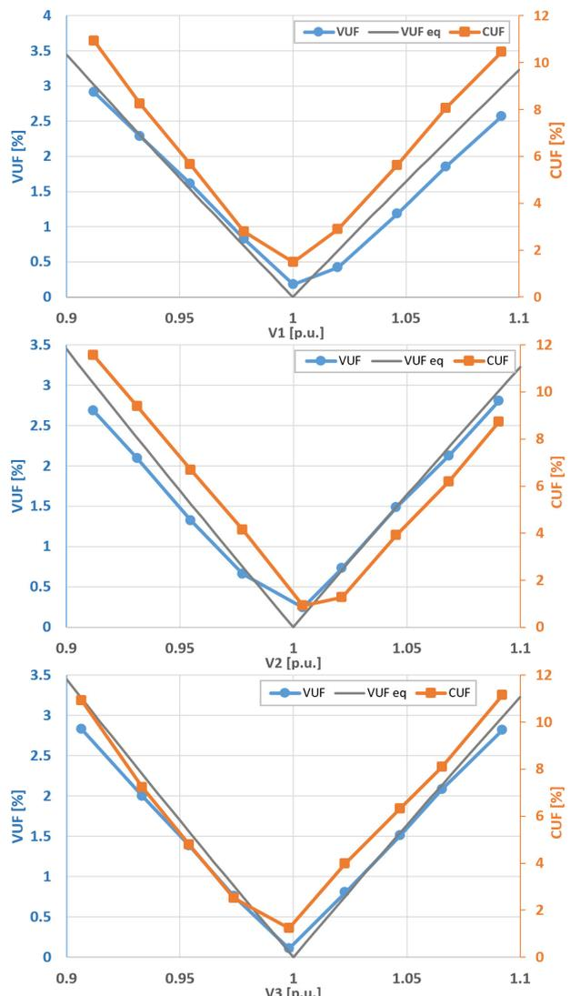
**Fig. 3.** *VUF* and *CUF* at single-phase unbalance
