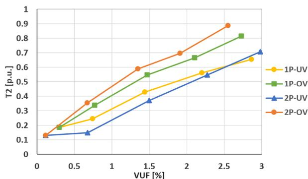
Fig. 6.  $T_2$  at single-phase and two-phase unbalance
