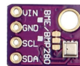
Fig. 3. BME280 multi-sensor board
