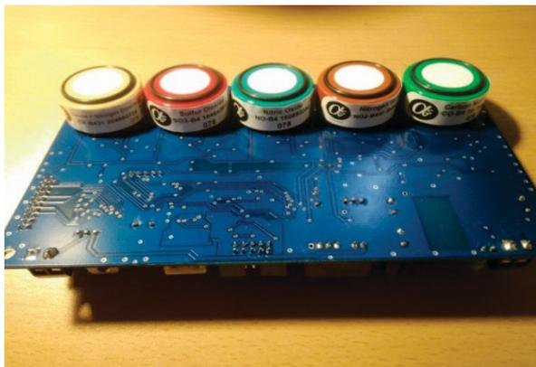
*Figure 1. A prototype of a multi-sensor gas-sensing head*
