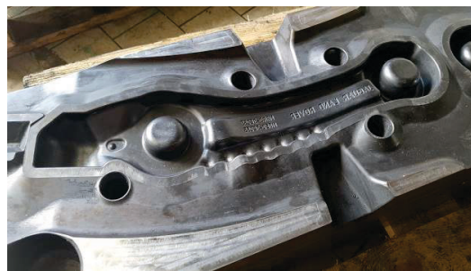
Fig. 2. A typical example of forming tools processing. Laser hardening can increase service life by up to 50%.
