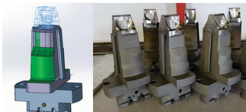
Fig. 4. Additively manufactured functional mold for aluminum die casting with internal channel structure
